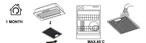
**Aluminium filters:** To avoid fires, clean thoroughly once a month or whenever the display pilot light lights up (if fitted). To do so, remove the filters and soak in hot water and detergent for an hour. If using a dishwasher, position the filters vertically to improve the cleaning process.
