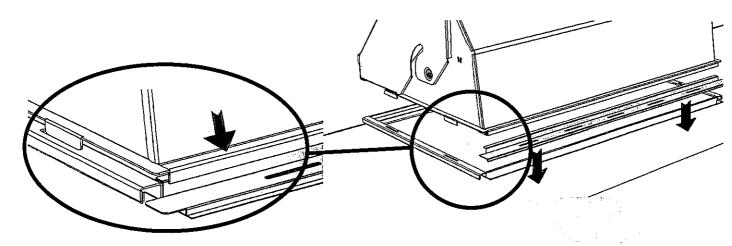
3. Pull Fat-Tray out half way, and attach the handle to place with 2 small screws and 2 nuts:
