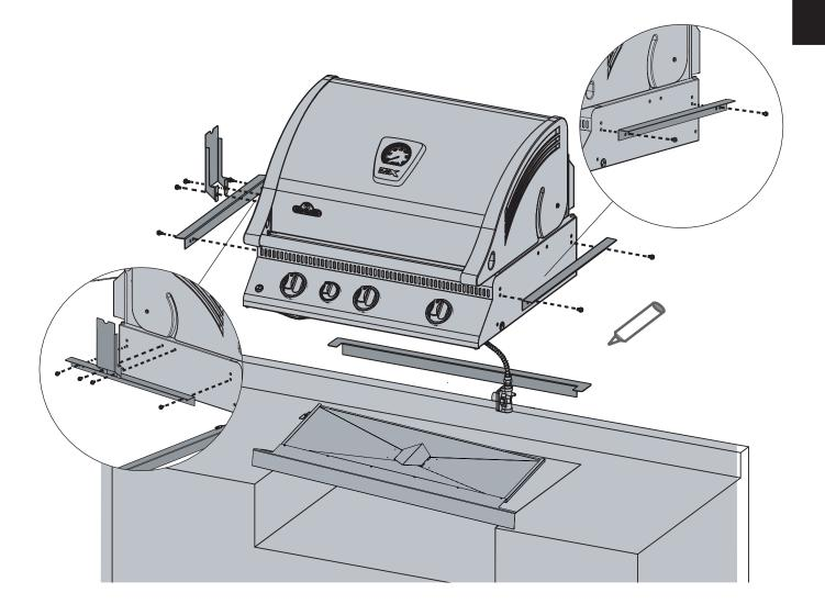
This grill is designed for masonry, **NON-COMBUSTIBLE** enclosures only and must be installed and serviced by a qualified installer to local codes.
