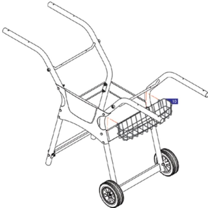
The condiment tray hooks onto the front of the "side middle panel".
