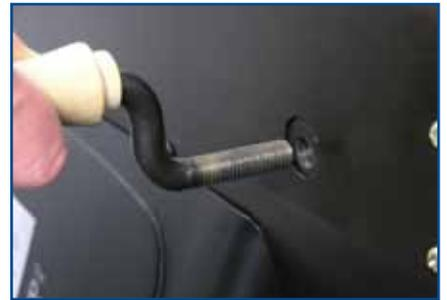
Oil/Grease the screw thread on the handle prior to fitting with 3 in 1 oil.
