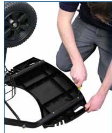
For ease of fitting use an electric screwdriver with the BarbeSkew legs upside down. Ensure the plastic tables are protected from being scratched when screwing upside down. The screws holding the tables to the legs should be fully tightened.
