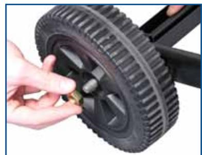
Please ensure the wheels are screwed in the correct way round (with the slight hump on the inside)
