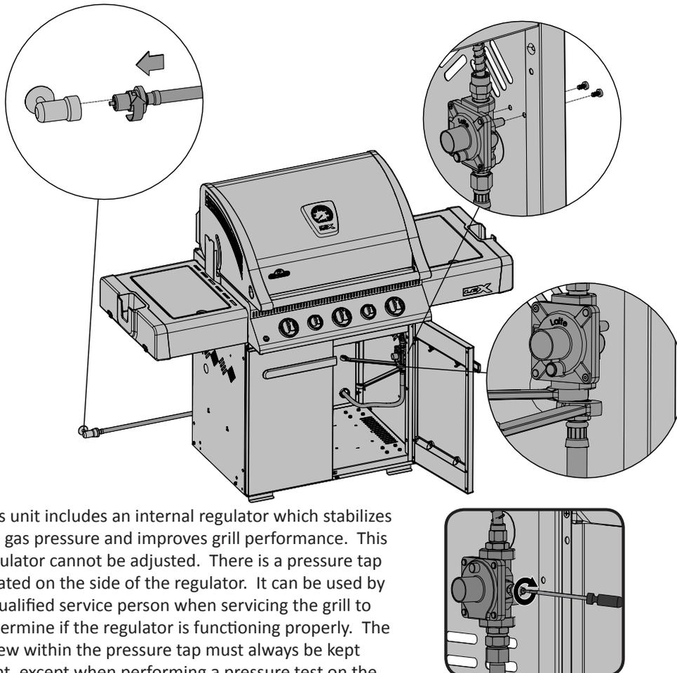
This unit includes an internal regulator which stabilizes the gas pressure and improves grill performance. This regulator cannot be adjusted. There is a pressure tap located on the side of the regulator. It can be used by a qualified service person when servicing the grill to determine if the regulator is functioning properly. The screw within the pressure tap must always be kept tight, except when performing a pressure test on the regulator (qualified service personnel only).
