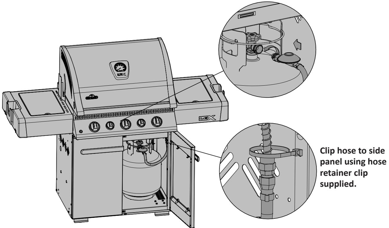
Ensure the regulator drops into the small opening, between the tank heat shield and the right side of the cabinet.
