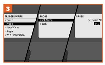
Press MENU; then scroll and select PROBE. You will be prompted to set a probe alarm for the internal goal temperature. Select SET ALARM. Then, at the probe menu, use the Selection dial to choose the temperature goal for your meat.
