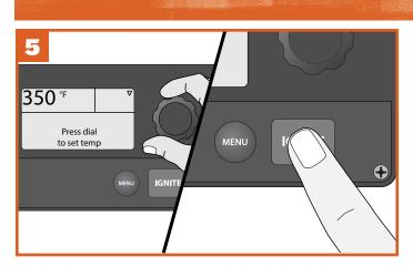
The home screen will display "Press dial to set temp." Turn the Selection dial clockwise to 350°F (I77°C). Press IGNITE, close grill door, and run grill for 20 minutes once it has reached the set temperature.
