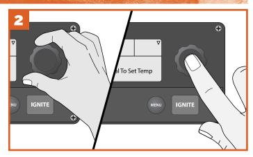
To select temperature, turn Selection dial right or left; once desired temperature is displayed, press the center of the dial to select.
