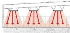
Radiant heat is directed downwards to where it is required, and can be zoned to heat only those areas that are occupied.
