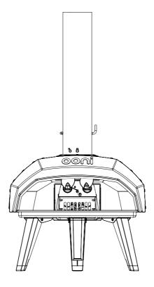
If Gas Burner for Ooni Karu 12 does not light turn the gas OFF and wait 5 minutes before proceeding to the next step. Always close the gas valve AND turn the button off during the 5 minute waiting period.
