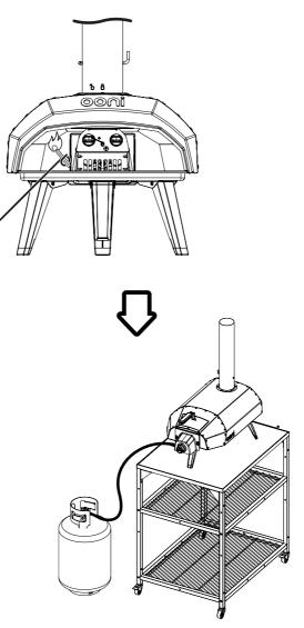
I Always route the gas hose away from the oven. The hose must not touch the oven body
